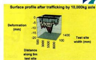
Fig 6. Deformation of the test pavement in the wheel track following trafficking by 10,000kg axles.
