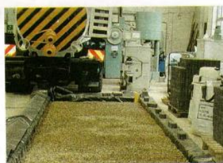
Fig 2. Open graded roadbase material installed in NUROLF.
